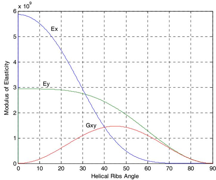
Fig. 8. Variation of elasticity modulus (GPa) versus ( $\varphi$ )
