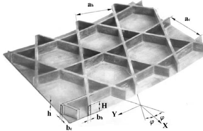
Fig. 2. Geometrical variables of a lattice plane:  $H$  = Height of cross-section of ribs (thickness of lattice layer),  $b_h$  = Thickness of cross-section of helical ribs,  $b_c$  = Thickness of cross-section of horizontal rib,  $a_h$  = Distance between helical ribs,  $a_c$  = Distance between horizontal ribs,  $\varphi$  = Angle of helical ribs with axis ( $x$ )
