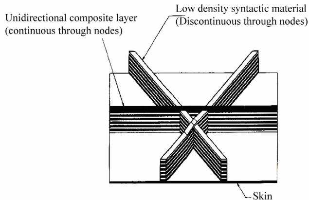
*Fig. 1. Joint points of ribs [5]*
